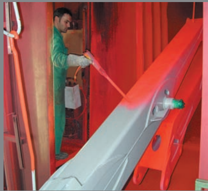
Powder coating with burn-in process at 200°C
