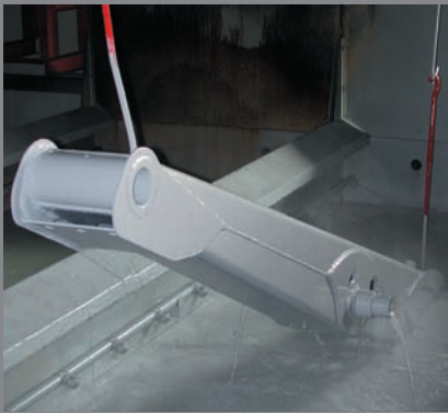
KTL-coating with burn-in process at 160°C
