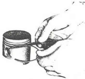
Measuring the clearance between piston ring and ring groove
