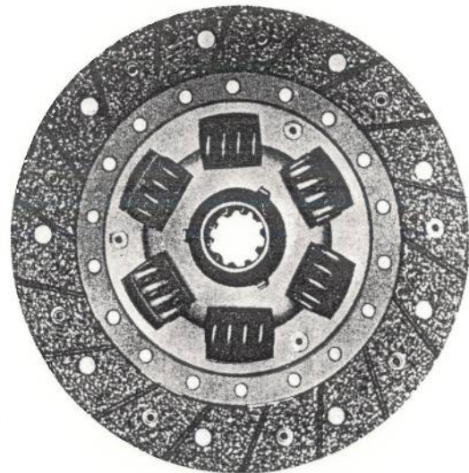
Assessing the serviceability of the clutch facing
