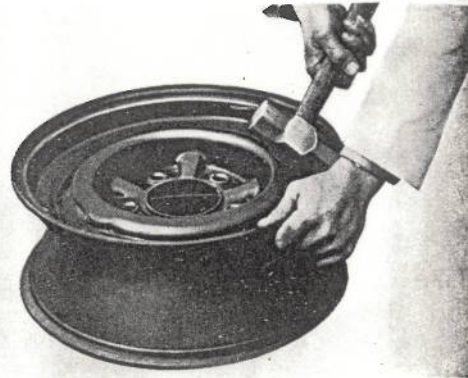
Reconditioning the rim flange
