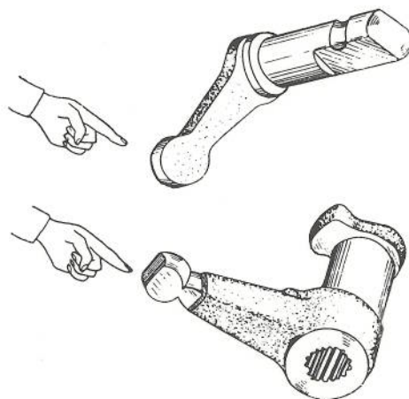
Checking the spherical ends of the internal shift lever and internal select lever
