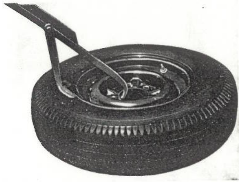
Removing the tire
