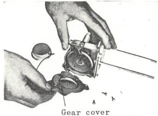
Removing the gear box cover
