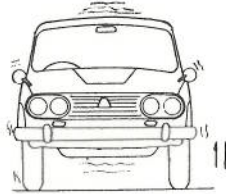
Out of static balance
