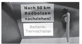
Battery circuit breaker Position of the battery circuit breaker
