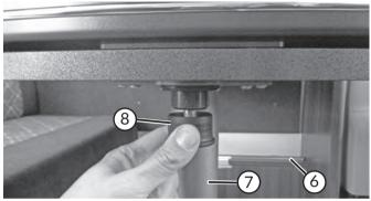
Locking pin underneath the table top
