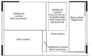
Rearranging the cushions Optima T65 GE with an L-shaped seating arrangement
