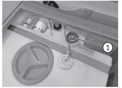
Outlet valve for fresh water tank
