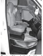
Footwell insulation in driver's cab Footwell insulation
