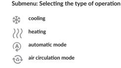
The type of operation can be changed using the "+/-" soft keys on menu bar C or by turning the jog wheel. The new selection must be confirmed by pressing the jog wheel or by means of the "On/Off" soft key.
