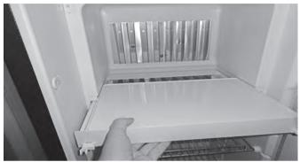
Removing the base of the freezer
