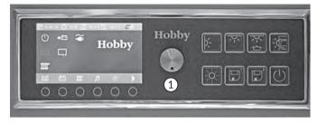
The system consists of control electronics, a TFT control panel with a keypad and several peripheral panels. It enables you to operate the different lights and several 230 V devices. Furthermore, various kinds of information and measured values are shown on the TFT display.
