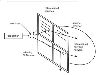
The overall system should allow simultaneous use of different models. Figure 6.1 presents an approach in which the PHB class is selected based primarily on the requirements of the application. Each class consists of several importance levels, emphasizing the need to have one unambiguous importance dimension inside the network, as described in section 4.5.2, "Importance," of Chapter 4, "General Framework for Differentiated Services."
