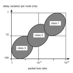
If the average load level is the only controlled factor, however, the relationship between delay and loss is not as clear as can be expected. Both low delay and low loss ratio can be achieved only if the traffic load is somehow controlled within a relatively short period, as described in the section "Priority Queuing" earlier in this chapter.
