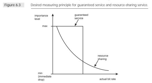
Note also that not only bit rate, but also packet rate can sometimes be an important factor. For a given link speed, the number of packets that the router has to handle each second depends on the packet size: The smaller the packets, the harder the processing requirement. Therefore, it can sometimes be reasonable to give more weight to small packets by using an extra term ( $B_0$ ), as shown in Formula 6.1.
