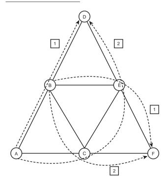
The main reason to use alternative routes is *load balancing*, which is a part of the larger problem of long-term network planning, in which the operator tries to optimize the use of network resources. Load balancing can be defined as the capability to decrease the maximum load by changing the traffic from links with high load to links with lower load. Remember, however, that the average load level is increased.
