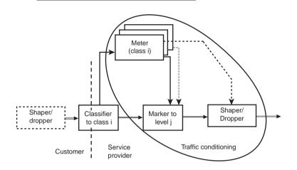
Moreover, based on the classification and marking result, the network can either delay some packets (that is, shape the traffic flow) or even drop packets. Nevertheless, it often seems more reasonable, for reasons discussed later in this chapter in section 6.1.4, "Traffic Shaping," to shape the traffic flow before metering and marking, perhaps in the customer's network.
